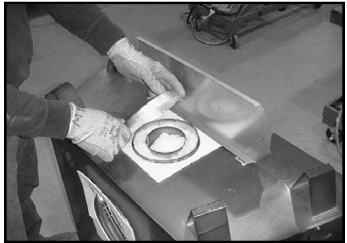
Figure 6.4 Remove the seal cap.
